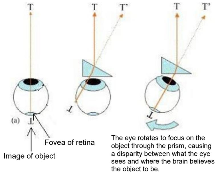
Figure 1b. Actions of goggles on light entering the eye
